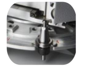
The special Protech tool holder eliminates the need to change tools for all multi-cutter processes that require changeovers, which are fully automatic on Protech.
