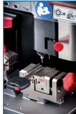
Laser and dimple key cutting station
